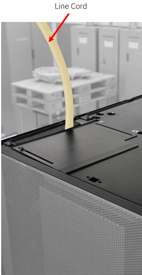
Figure 3: Top Exiting Line Cord without an Enclosure (FC 7803)
