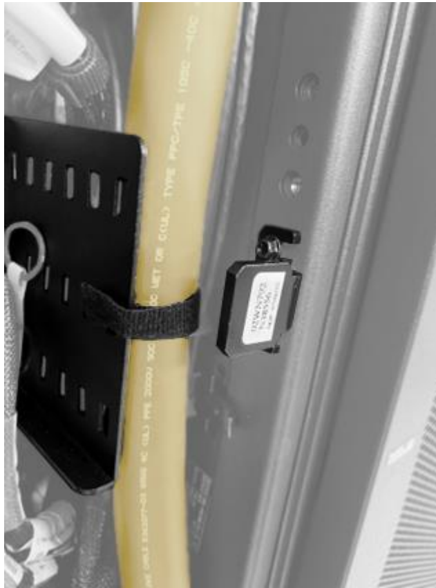
Figure 7: Use hook and loop to retain line and cord and keep away from latch
