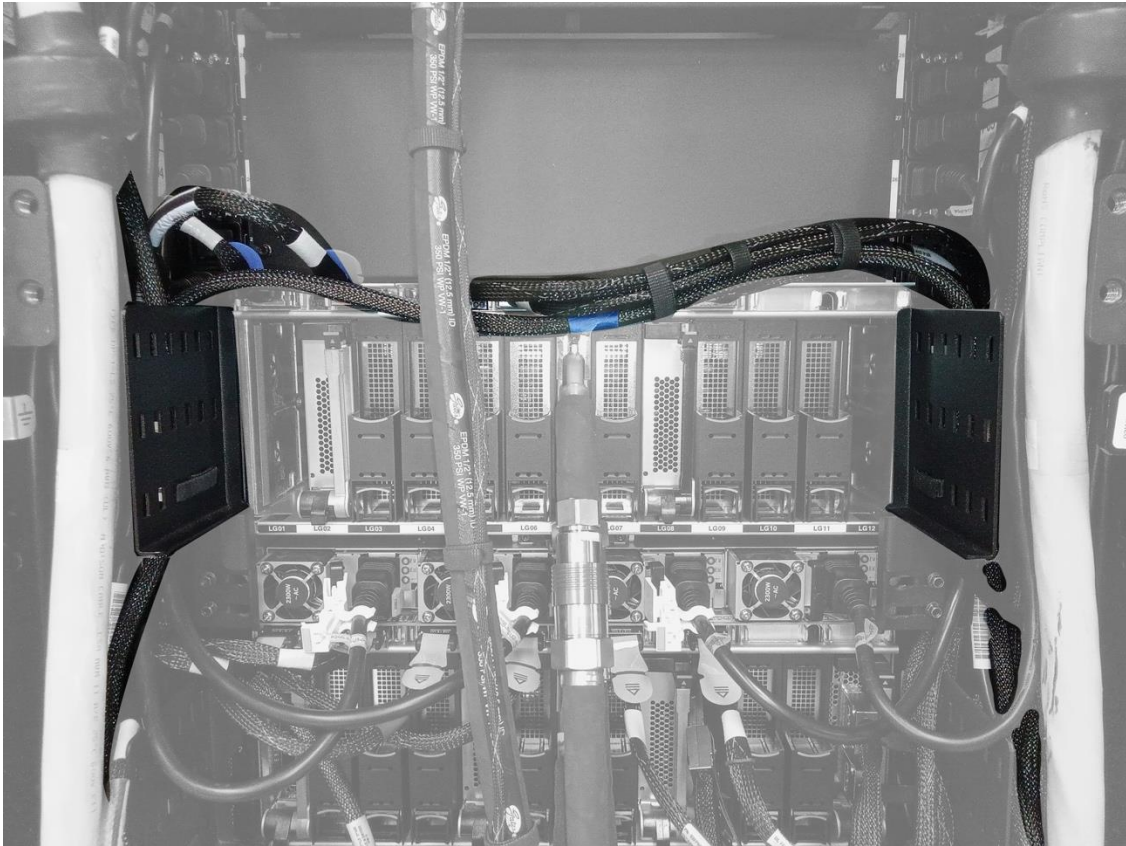
Figure 37: PCIe+ I/O cables Routed Across A-Frame
