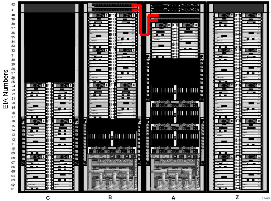
Figure 28: B to A Frame Ethernet Cabling through hole #1
