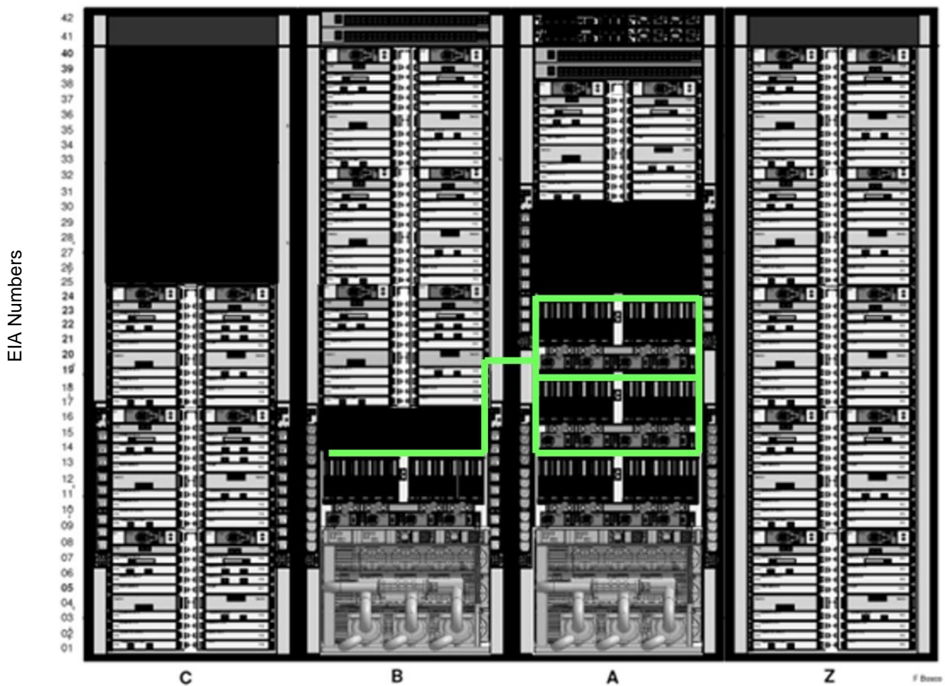
Figure 33: SMP Cabling through hole #3
