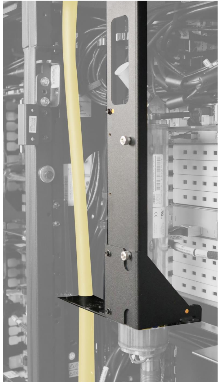
Figure 2: Line Cord routed behind Reservoir Bracket
