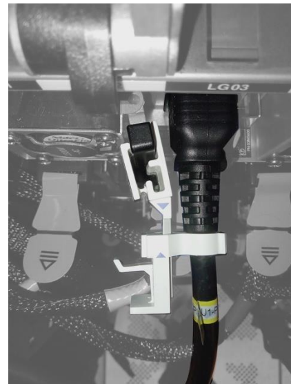
Figure 18: Large PSU Clip fully installed
